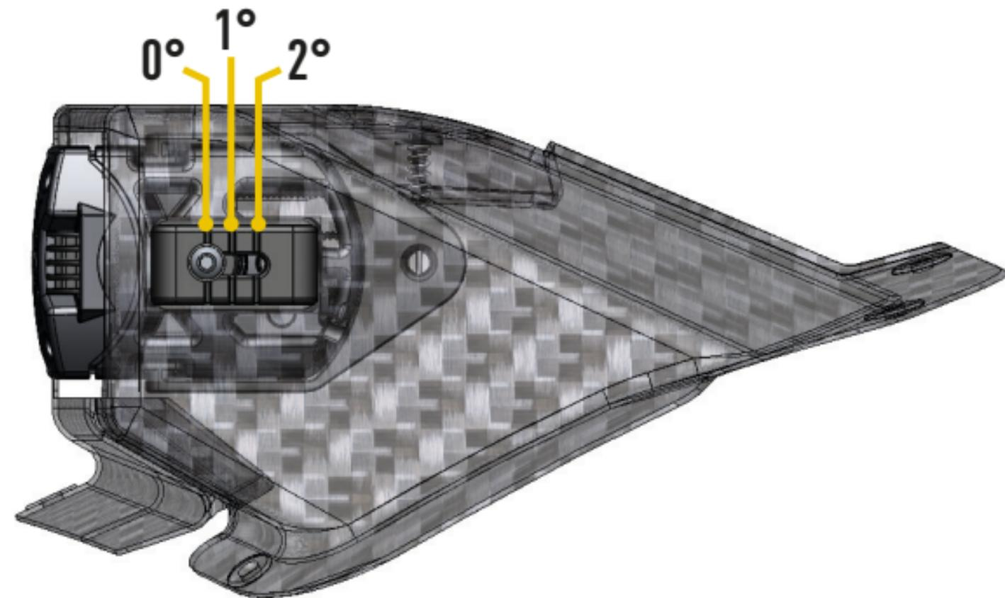
\* LOOSEN OUTBOARD SIDE MOUNT SCREW BEFORE ADJUSTING. UP/DOWN ADJUSTMENT +/- 5°
