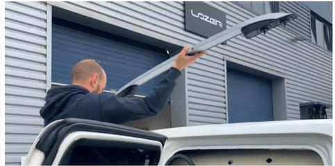
3. Having ensured sufficient structural integrity in the roof rail, mark and drill 5mm rivet holes (through roof rail and/or cover plus any support material behind - support material is not supplied in this kit).
