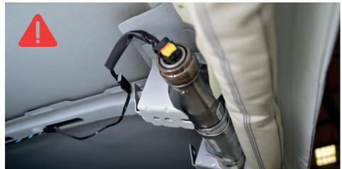
7. Having prepared the surface areas with the supplied VHB cleaner pad, apply sealant to ensure a sealed cable entry both into the roof rail, and into the headlining.
