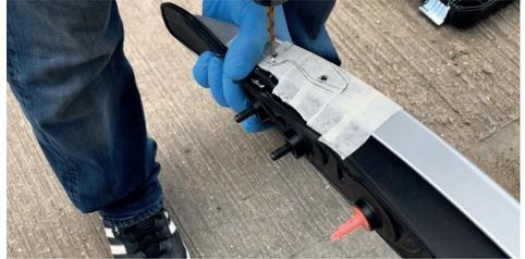
4. Considering preferred cable route into roof rail, mark and drill a 9mm cable entry hole (on the left-hand roof rail). Identify and remove material which might otherwise restrict cable entry, or routing through into vehicle headlining. File any sharp edges.
