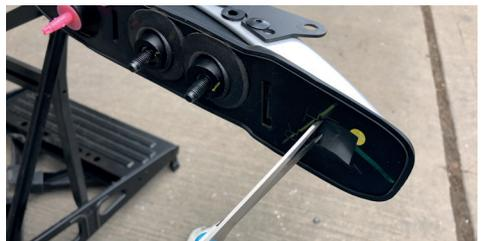
5. Having removed the relevant connector from either the lamp or wiring harness (to facilitate routing through the roof rail/roof), feed the cable grommet(s) through the cable wire.
