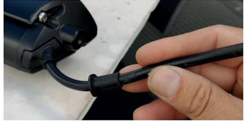
6. The connection to the wiring harness can be made within the roof rail (space permitting), or within the roof lining. Drill a 9mm hole in through the roof rail and vehicle roof for the cable routing into the vehicle's headlining. CAUTION – Take care to avoid interference with any air-bag systems on the vehicle.
