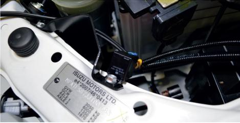
For vehicles that do not produce a constant 12v signal from the back of the headlight will require a CanM8 High Beam interface to control the signals. Please see our youtube channel, or scan the QR code for more information regarding install of the CanM8 interface.
