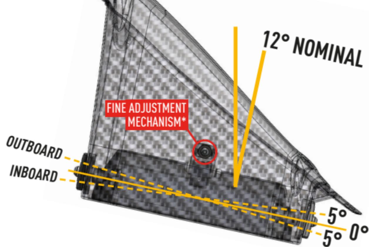
\* LOOSEN OUTBOARD SIDE MOUNT SCREW BEFORE ADJUSTING.
