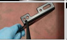
Apply sealant to the underside of the brackets to create a watertight seal.
