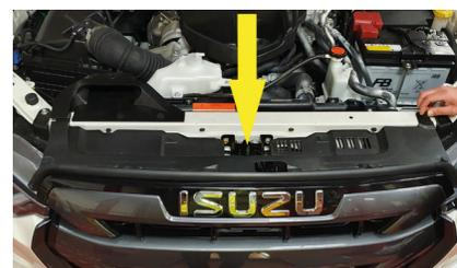
Carefully insert the lamp assembly into position behind the centre grille.
