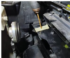
Mark out where the end brackets need to be drilled and drill a 6mm hole.
